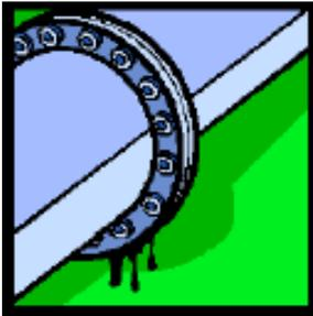
Failures in FRP pipe generally result in a weeping leak that can easily be repaired. HDPE failures are typically catastrophic and repairs generally are difficult requiring special fusion equipment. Special fittings, modification to piping systems, etc. all of those difficulties usually experienced in construction of a plant are easily accommodated in FRP.
