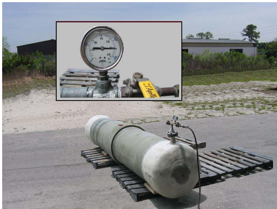
In house testing of our 24" diameter single o-ring joint was done to 250 psi with no leaks.
