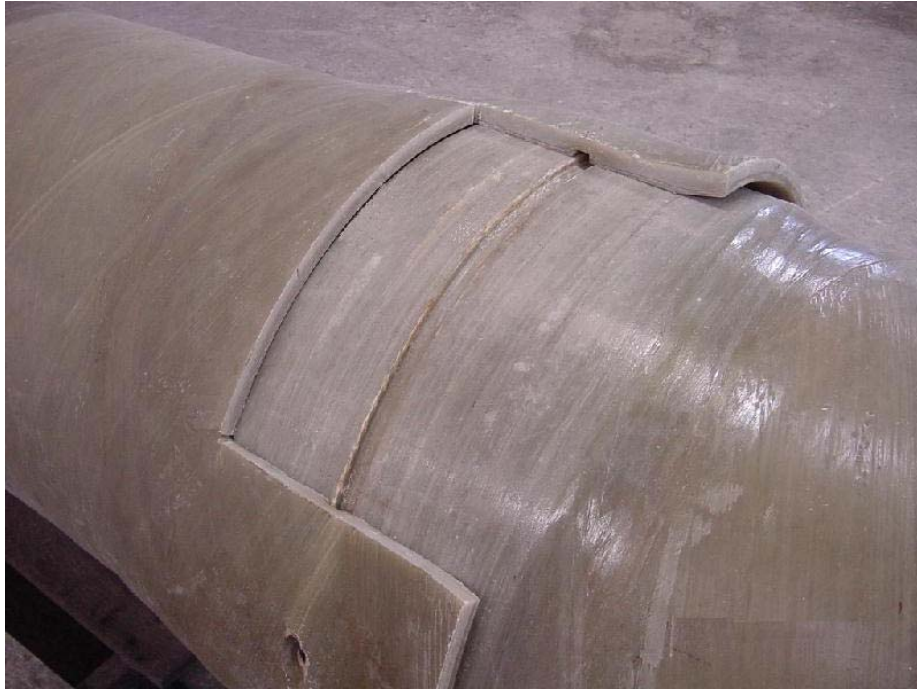
24" diameter prototype joint, after high pressure testing - This joint was cut away to examine the grooves and laminate for stress assessment
